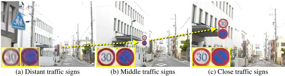
Fig. 2. Appearances observed at distant, middle and close traffic signs from a vehicle
