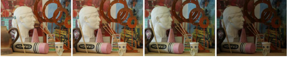
Fig. 1. Illumination and exposure differences for the Art [14] input pair. Left to right: left (base) reference image, and right (match) image with identical illumination/exposure, right image with illumination change, right image with exposure change.
