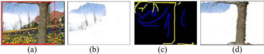
Fig. 4. Results using GrabCut. (a) The initial input is a red rectangle. (b) Result after drawing the rectangle. (c) The additional inputs are some scribbles, in which the yellow scribbles indicate the foreground and the blue scribbles indicate the background. (d) Result after applying those scribbles.
