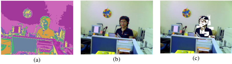
Fig. 3. (a) Watershed segmentation result; (b) KLT feature points; (c) extracted foreground regions following watershed segmentation and KLT feature point extraction
