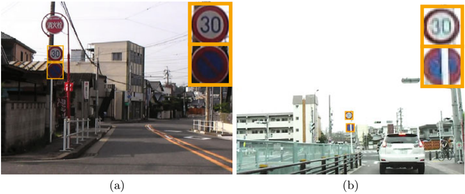
Fig. 8. Examples of detection results by the proposed method (LRP). (a) there is an object similar to the target traffic signs, which is located above the traffic signs but correctly not detected, and (b) although a traffic sign is occluded by a pole, the proposed method succeeded to detect it.
