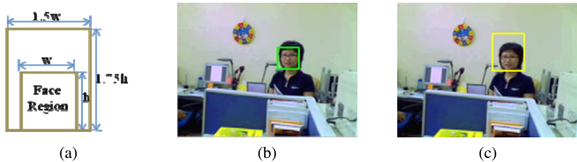
Fig. 5. (a) ROI template; (b) the face detection result is circumscribed by a green rectangular; (c) the corresponding ROI for protruding object detection is circumscribed by a yellow rectangle
