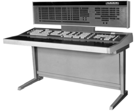
Fig. 4. Super-computer “Almaz” engineering control console
