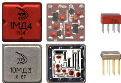
Fig. 7. First series IC in the USSR, “Tropa”, thick-film, a top number, “Posol”, thin-film, the bottom number. (At the left and in the center – in the double size, on the right – in full size).
