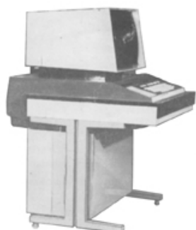
Fig. 2. The device of visual display (UVO). The symbolical display. Diagonal of the screen (43 cm); Size of the screen (220x200 mm); Symbols (up to 2048); Lines on the screen (32); Symbols in line (64); Size of a symbol (3.5x2.5 mm); Ensemble of symbols (128).
