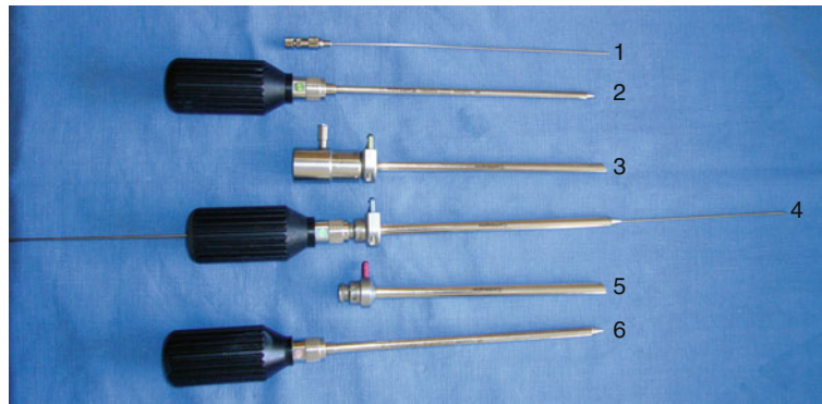
Fig. 11.10 Photograph of a modular cannula system (Arthrogarde hip arthroscopy cannulas, Smith and Nephew, Andover, MA). (1) Hip arthroscopy needle (spinal needle). (2) Cannulated obturator for the 4.5-mm modular cannula ( green color coded for the 4.5-mm obturator–cannula assembly). (3) 4.5-mm modular hip arthroscopy cannula. Note a single inflow irrigation extender is attached to the modular end of the cannula. The irrigation extender
