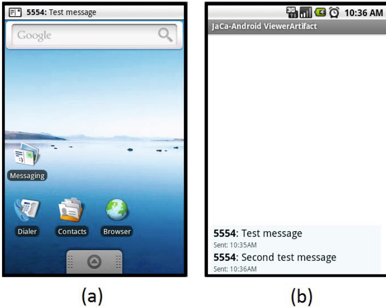
Fig. 2. The two different kinds of SMS notifications: (a) notification performed using the standard Android status bar, and (b) notification performed using the ViewerArtifact
