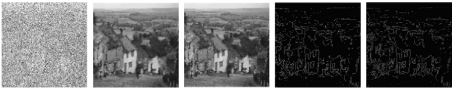
Fig. 7. First figure is the Goldhill image corrupted by the Noise Model 4(20% salt ,60% pepper),second and third figure shows the images restored by MNASM and NAWSM filter respectively and fourth and fifth figure shows the corresponding edge maps (obtained by using Sobel operator).
