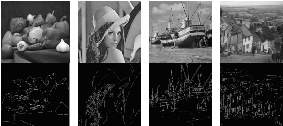
Fig. 1. The First row shows standard test images Peppers, Lena, Boat and Goldhill used for performance evaluation of our proposed NAWSM filter. The second row shows their edge maps obtained by Sobel operator.
