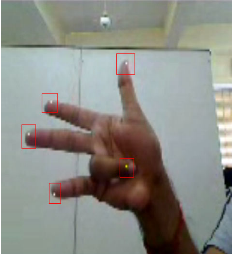
Fig. 3. Fingertips and Center of palm detected in the extracted image
