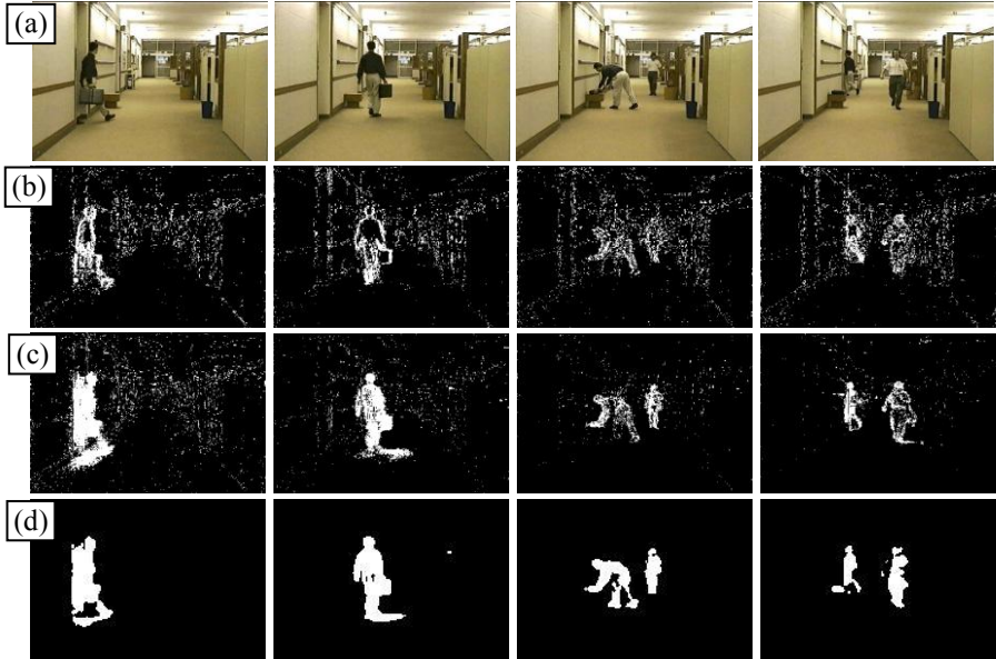
Fig. 2. Background subtraction results on Video 2 (Hall Monitoring) a) Original frames. b) Frame differencing results c) IGMM results d) Proposed method results
