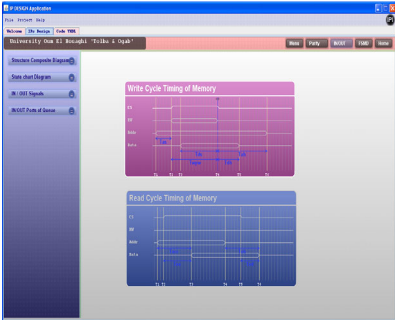
Fig. 4. Memory write and read operations modeling using Timing diagrams
