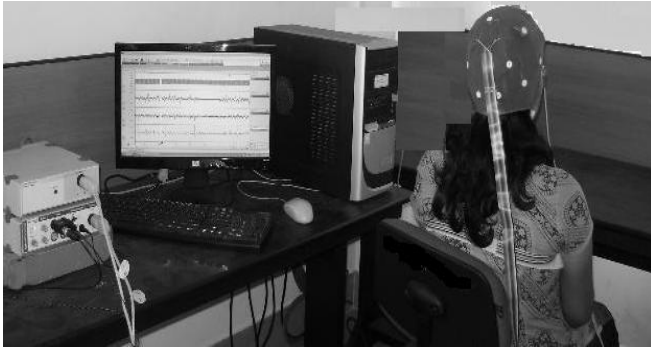
Fig. 1. The experimental setup: A subject, performing tasks, with the Electro-Cap for EEG recording
