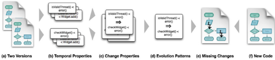
Fig. 2. How LAMARCK works. Given two versions (a), LAMARCK extracts temporal properties (b) that characterize object usage in each version. The differences (c) are then mined for recurrent change patterns (d). These patterns can then be used to search for missing changes (e) in new code (f).
