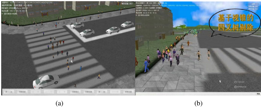
Fig. 4. (a) City block crowd was simulated with the 64×64 coarse grids. (b) When we pause the simulation and move the spectator around, it will be seen that there is no agent out of the sight. Which means our method simulates a few agents of the crowd and reduces the cost of both updating agents’ states and computing their interactions.
