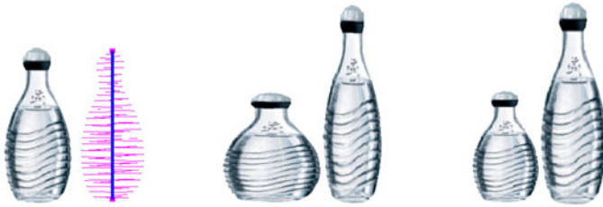
Fig. 3. Deformation with (middle) and without (right) global area preservation. The original object and variable-length needle model are shown on the left.
