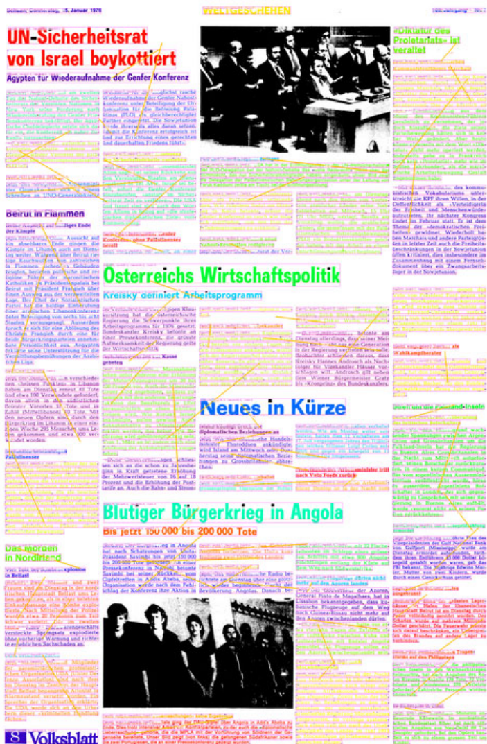
Fig. 12.5 Example of MST-based article segmentation on a newspaper image: result after the extraction of the Minimum Spanning Tree.
