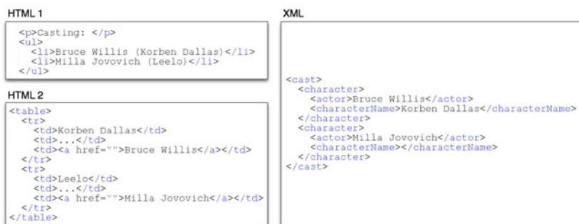
Fig. 13.1 Example of web page wrapping. This is a case of XHTML to XML Structure Mapping. Nodes can be relabeled, inserted, suppressed and moved.
