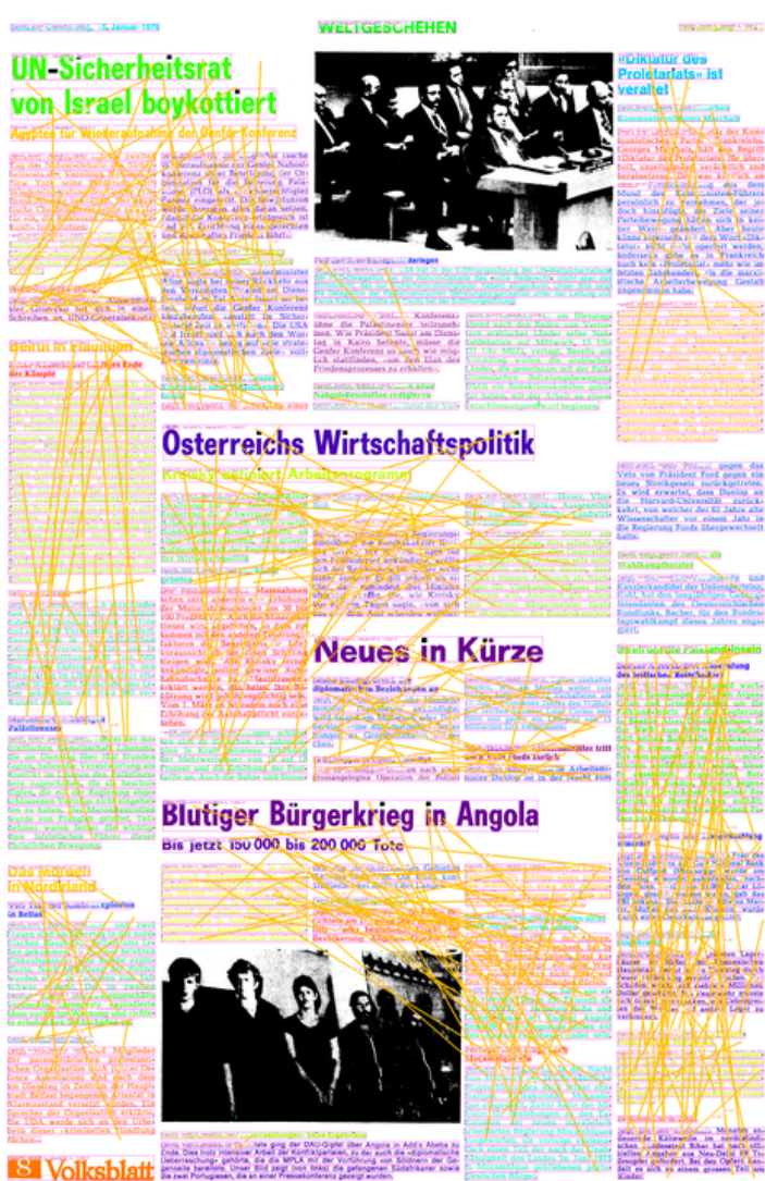
Fig. 12.4 Example of MST-based article segmentation on newspaper image: initial graph edges.
