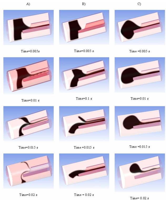
Fig. 3 Snap shots of clot absorption when time progresses, for the three cases of A) early clot, Newtonian, viscosity 0.035 Pa·s, no surface tension; B) late clot, Newtonian, viscosity 0.6 Pa·s, no surface tension; C) Newtonian, viscosity 0.035 Pa·s, surface tension 0.1 N/m
