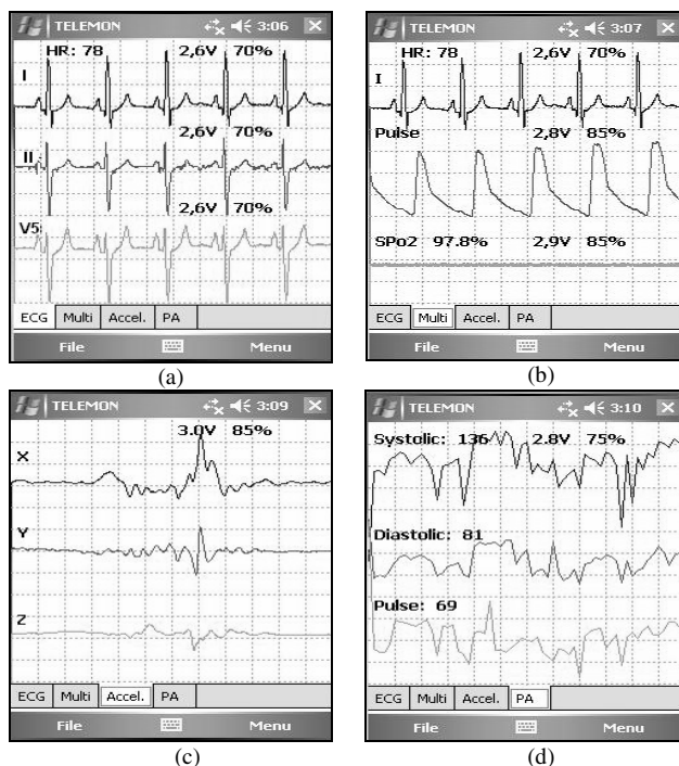
Fig. 4 The Personal server interface: (a) 3 ECG traces, (b) one ECG trace, pulse waveform and SpO 2 , (c) 3 accelerometer traces, (d) systolic, diastolic pressure and pulse diagrams, measured each 30 minutes
