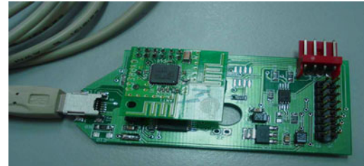
Fig. 9 Prototype hub device connected to USB port
