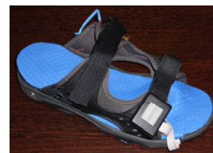
Fig. 8 Prototype shoe with in-sole device and warning device
