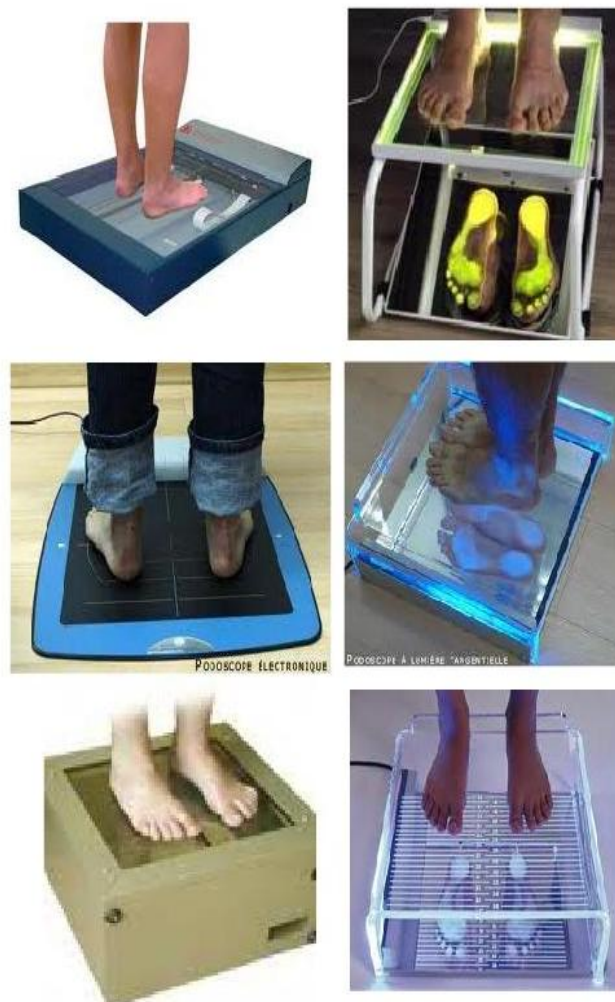
Fig. 2 Podoscope types: analogue with mirror and side illumination, structured visible lighting, optical scanner, capacitive sensing, camera based acquisition
