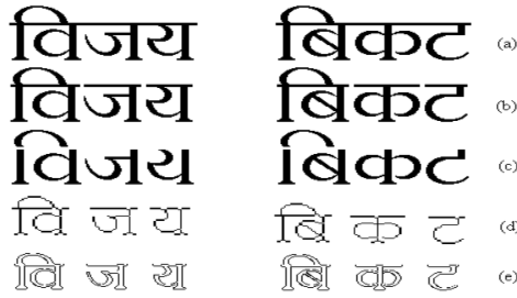
Fig. 1. Preprocessed Images (a) Original, (b) segmented (c) Shirorekha removed (d) Thinned (e) image edging
