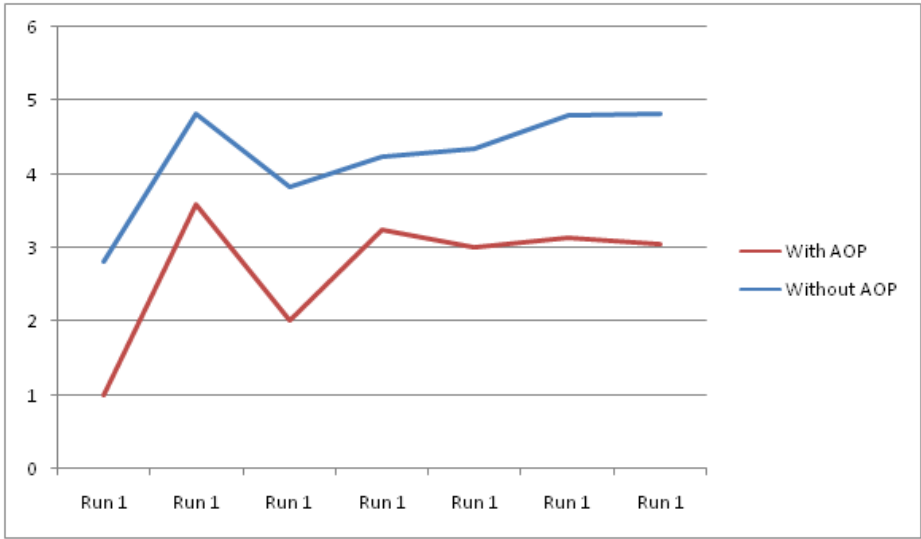
Fig. 4. Execution time analysis for Web Service Calling without AOP and with AOP
