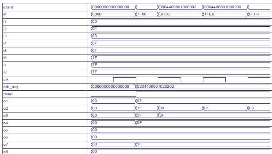
Fig. 7. Simulation waveform of 8 x 8 Switch
