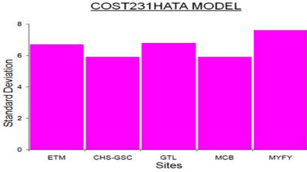
Fig. 7. Standard Deviation Of Prediction Error Of Path Loss Of COST231Hata Model
