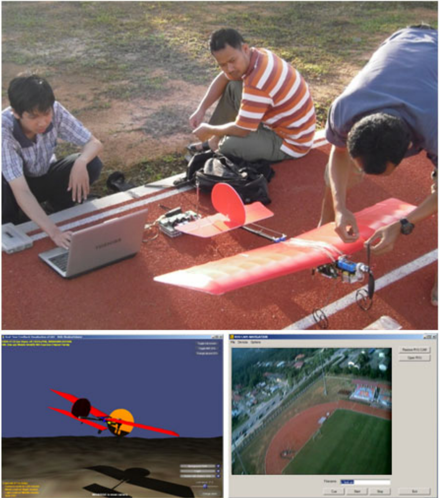
Fig. 5. Testing of Red Glide with geo-mapping and visual 3D Feedback
