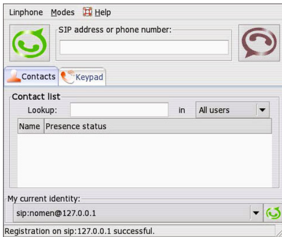
Fig. 6. Successful registration of a SIP VoIP client
