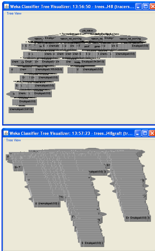
Fig. 3. The top figure is the tree structure for J48 and the bottom figure is the tree structure for grafted J48. Grafting adds nodes to the decision trees to increase the predictive accuracy. In the grafted J48, new branches are added in the place of a single leaf or graft within leaves.
