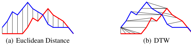
Fig. 1. The two time series (top blue and bottom red curves) show the same pattern shifted along the time axis; Euclidean Distance (vertical lines) does not capture this, whereas DTW aligns time series and computes the distance between the best match
