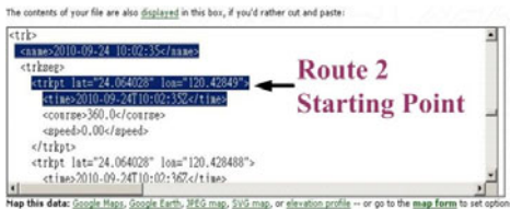
Fig. 7. The 2 nd route shown on Google Map indicating the latitude, longitude, and the time stamp of the starting point
