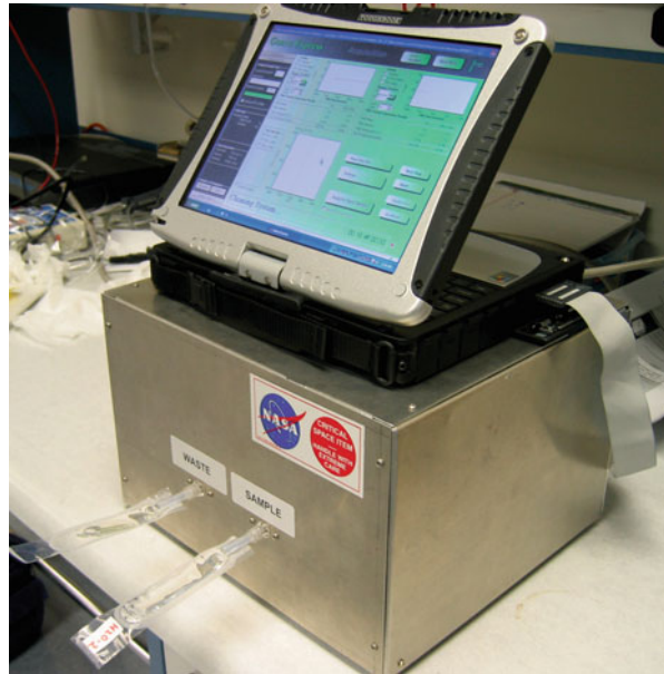
Fig. 24.5 NASA-JSC prototype flight cytometer with sample delivery WBSD units affixed to the sample delivery ports
