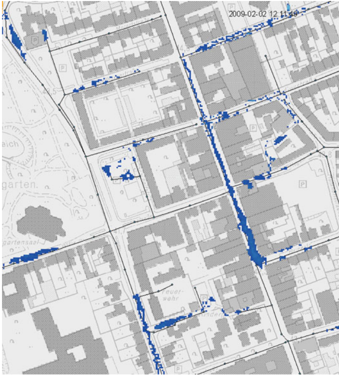
Fig. 10 Flooding after a rainfall event with a return period of five years—Herne-Wanne
