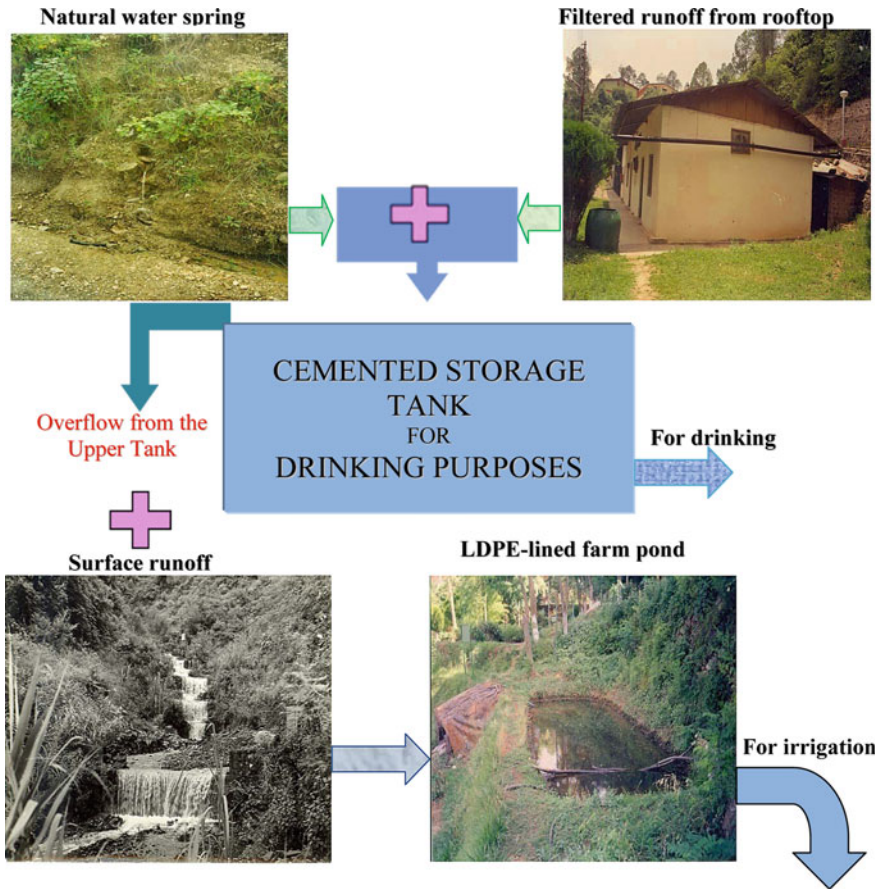
Fig. 5 Appropriate water harvesting model for hilly areas
