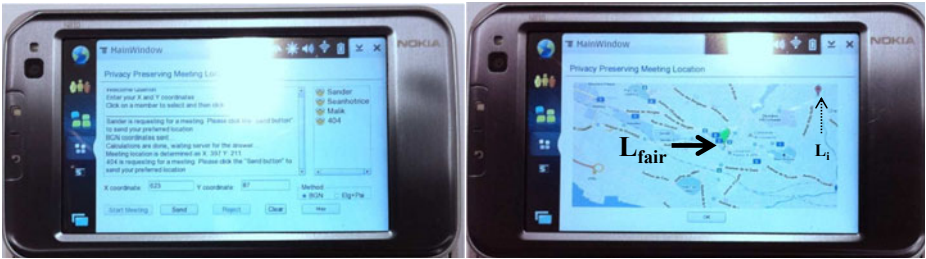
Fig. 4. Prototype PPRFVP application running on a Nokia N810 mobile device. The image on the left is the main window, where users add the desired meeting participants. The image on the right is the map that shows the fair rendez-vous location (green pin) and the user-desired rendez-vous location (red pin).
