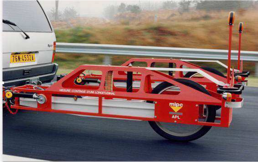
Fig. 5.8 Longitudinal Profile Analyzer (APL in french)
