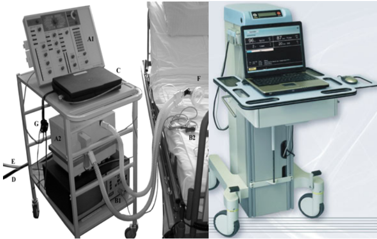
Fig. 3. The Automatic Lung Parameter Estimator (ALPE) system, in its research [5], and commercial (ALPEessential™) forms. (The research version is printed with kind permission from Springer Science+Business Media: J Clin Monit Comput , The Automatic Lung Parameter Estimator (ALPE) system: Non-invasive estimation of pulmonary gas exchange parameters in 10-15 minutes, 17, 2002, page 44, Rees SE, Kjærgaard S, Thorgaard P, Malczynski J, Toft E, Andreassen S, figure 1. The commercial picture is with kind permission of Mermaid Care A/S).
