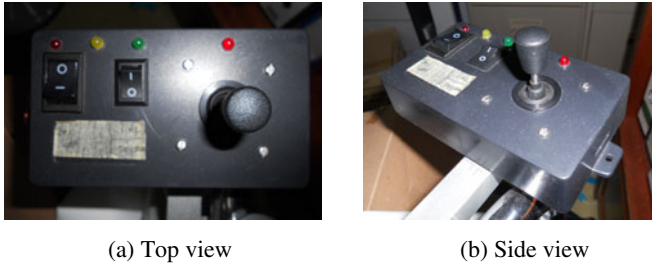
Fig. 2. Existing wheelchair controller mounted on a bar besides the right arm of the wheelchair
