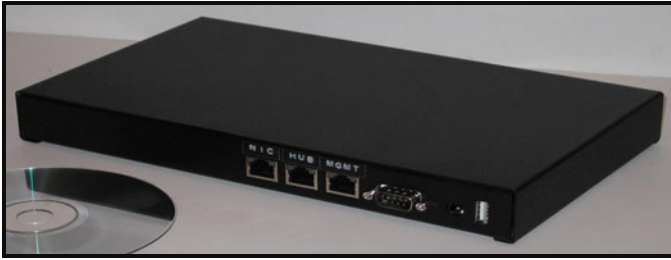
Fig. 2. The portable network forensic evidence collector [13]
