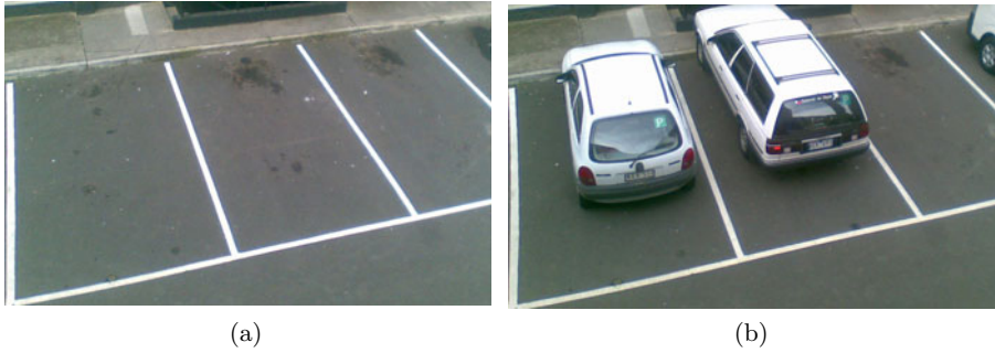
Fig. 1. (a) A reference image where the parking lot is empty. The same set of filter is applied to the reference image as well as the incoming image stream represented by (b). For images streams where the vehicle colour is light (as in (b)), it is rather easy to obtain a high detection accuracy.
