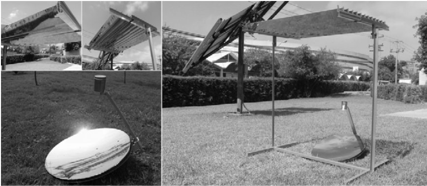
Fig. 9. Semi-passive solar concentrator prototype
