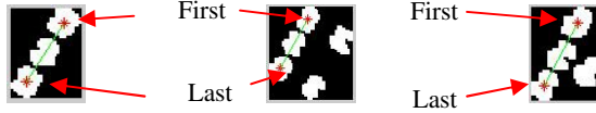
Fig. 9. Samples of detected Braille cells after localizing the center of first and last dots
