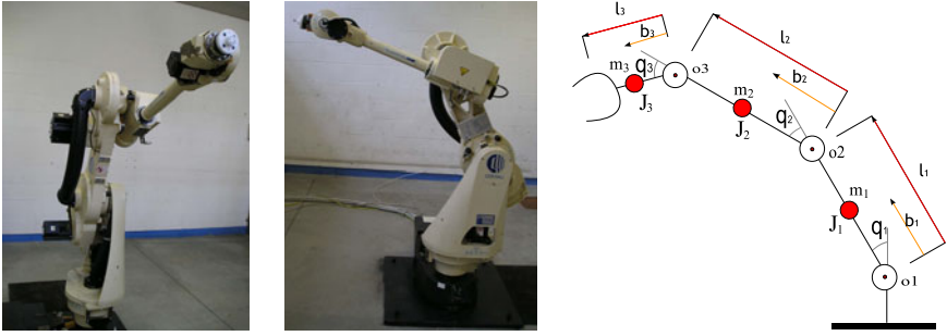
Fig. 20.2 The COMAU SMART3-S2 robot manipulator.
