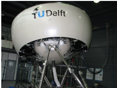
(b) SIMONA flight motion simulator (outside view)
