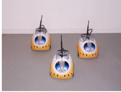
Fig. 15.8 The Pekee nonholonomic mobile robots.
