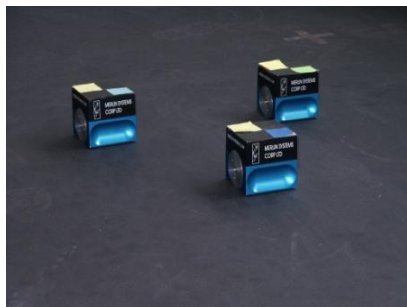
Fig. 15.11 The Miabot nonholonomic mobile robots.
