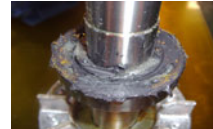
(b) Bearing fault
