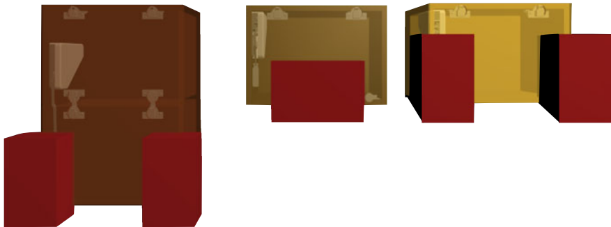
Fig. 3. Some haptic snapping effects have been introduced to simplify interaction with the Virtual Prototype. When the virtual hand is inside one of the red blocks it automatically changes its shape mimicking a real hand interacting with the same object and is attached to the door returning to the user forces and torques.
