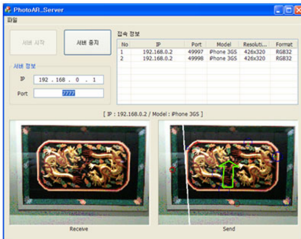
Fig. 4. An example of server-side operation. Left image is one received from iPhone. Right one shows the direction to the target location.
