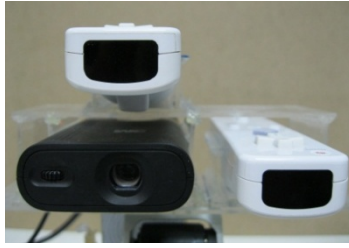
Fig. 5. Two Wiimotes attached closely on both horizontal and vertical axes of portable projector
