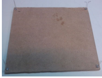
Fig. 3. Four diffusion infrared LEDs embedded on the corners of surface display
