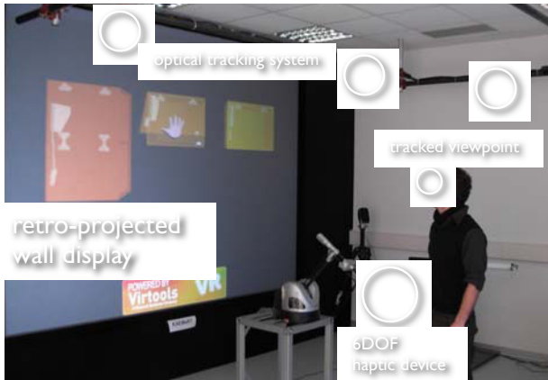
Fig. 2. The hardware setup used to implement the case study consisting in: an optical tracking system, a retro-projected wall display and a 6DOF haptic device equipped with a generic handle
