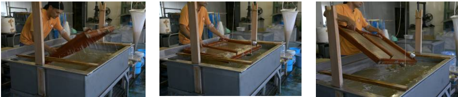
Fig. 1. Three main movements in Japanese papermaking; scooping, swinging and draining (from the left)
