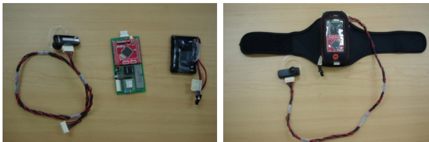
Fig. 2. The prototype device for the neck's posture detection
