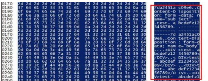
Fig. 3. Plain text packets passing through usual wireless LAN security system
