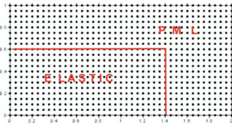
Fig. 6. Regular mesh with PML region
