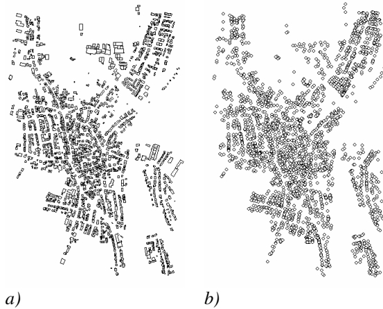
Fig. 5. (a) The ground polygon and (b) point shapefile of the Plieningen data set
