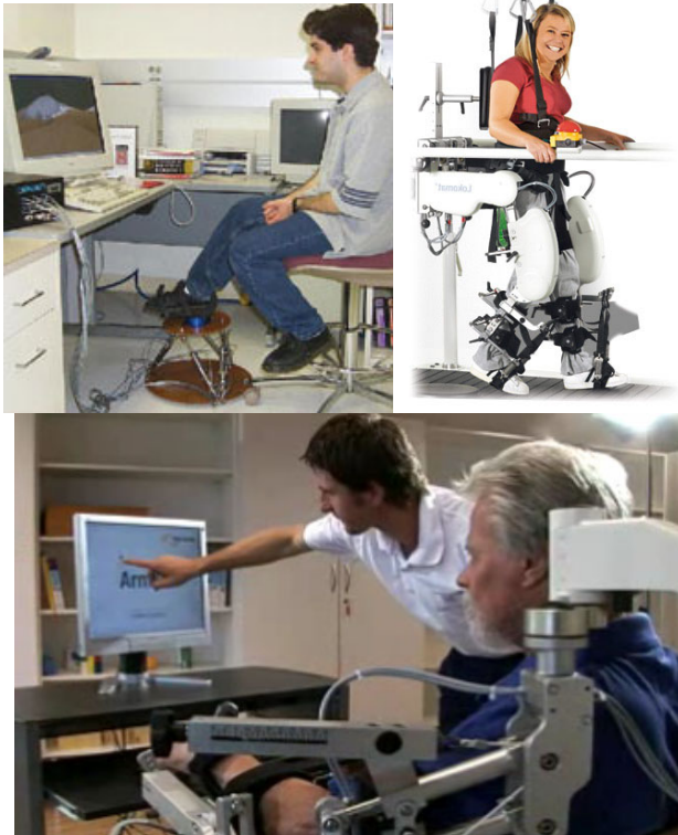
Fig. 1. Successful applied examples of technologies for rehabilitation. Up: Rutgers Ankle (on the left) and Lokomat ® (on the right). Down: Armeo ® .
