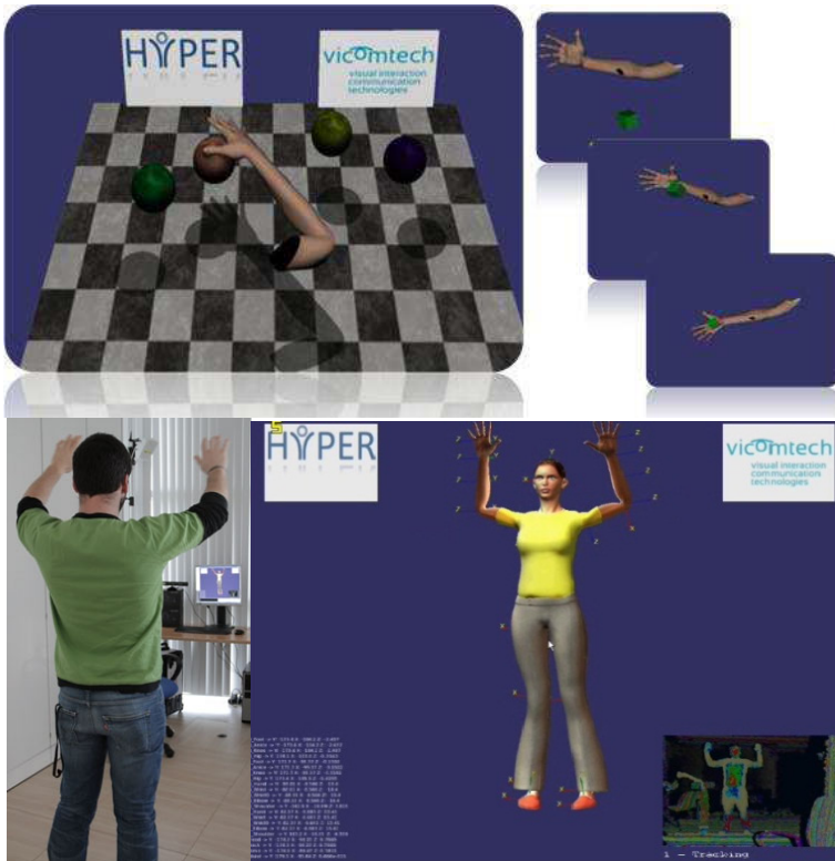
Fig. 2. Up: Snapshots of simple VR scenes: reaching, moving and grasping a virtual object. Down: tracking with Kinect®
