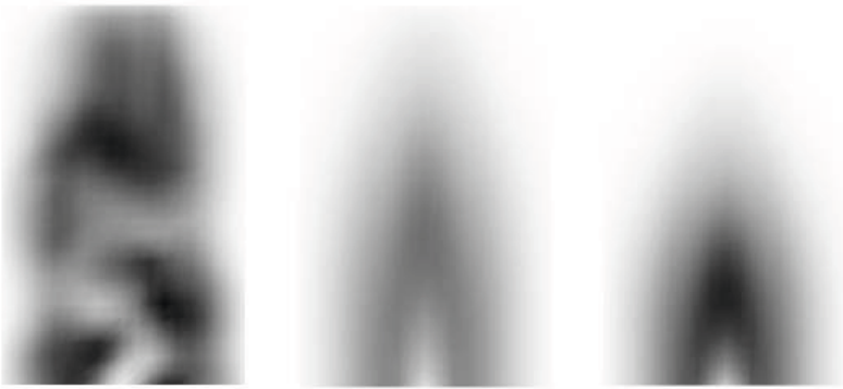
Fig. 2. The \text{CO}_2 density for lean, stoichiometric and rich methane-oxygen mixtures
