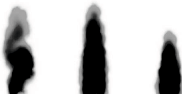
Fig. 4. The light radiation in gray scale for lean, stoichiometric and rich methane-oxygen mixtures. The black color corresponds to the strongest radiation.
