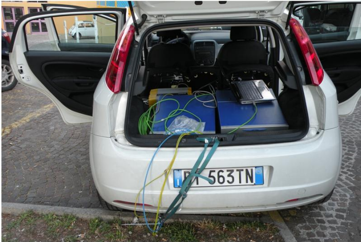
Fig. 6. AVL 483 Micro Soot Sensor mounted on the vehicle for the campaign acquisition
