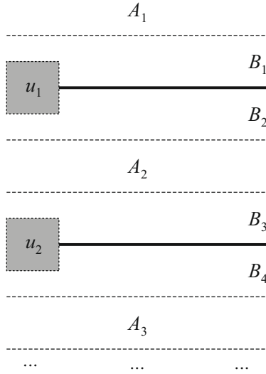
Fig. 2. Layout stripes: A_1, A_2, \dots — the stripes for layout of the secondary vertex labels; B_1, B_2, \dots — the stripes for layout of the edge labels
