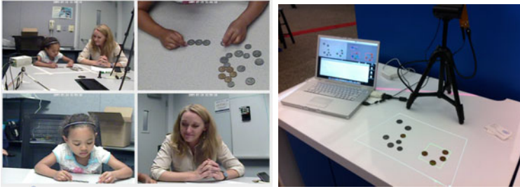
Fig. 1. Four video cameras simultaneously captured the interaction from four angles. The camera/projection system on the right, recognizes the clusters of coins and types within each cluster. In this instance it projects hints on a table to help the student separate the pennies from the rest of the coins.
