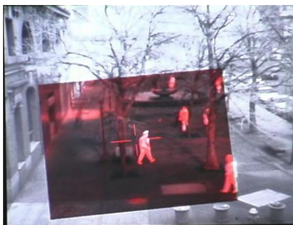
Fig. 2. Night REAPER augmented reality view. The grayscale background represents the intensified imagery, and the color overlay represents the imagery from the thermal weapon sight.
