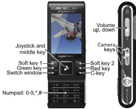
Fig. 1. The embedded device and its input keys
