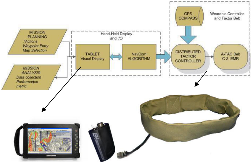
Fig. 4. Block diagram for the proposed ATAC-NavCom system
