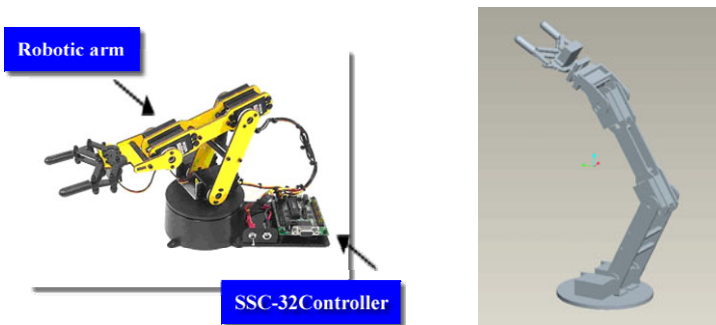
Fig. 3. Manipulation module: robotic arms image and its CAD model
