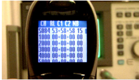
Fig. 3. Victim phone has camped-on to the fake base station
