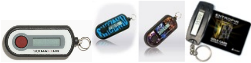
Fig. 2. Hardware Tokens: Square Enix Security Token (left), Blizzard (Battle.net) Authenticators (middle), and MindArk's Gold Card Kit for Entropia (right)
