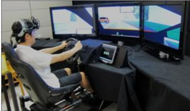
Fig. 1. The STISIM driving simulator and in-vehicle interface
