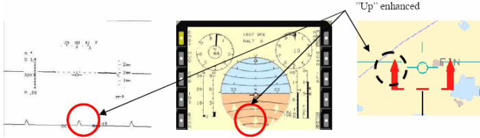
Fig. 3c. Attitude display (Consistency, Support of user mental models)
