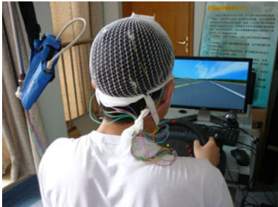
Fig. 1. The driving simulator and virtual driving scene
