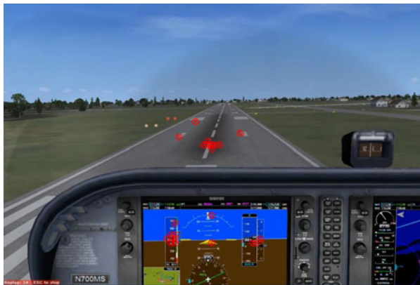
Fig. 2. Fixation Overlay on Approach (red circles indicate fixation points)
