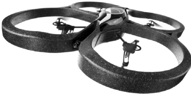
Fig. 1. AR Parrot drone protective enclosure [11]
