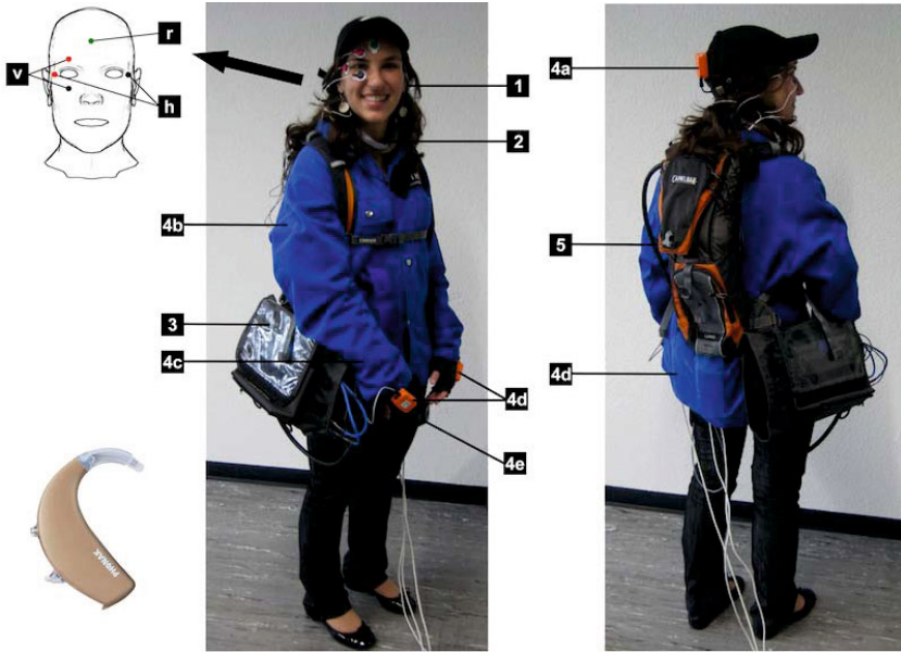
Fig. 6. Sensor setup consisting of HIs (1), a throat microphone (2), an audio recorder (3), five EOG electrodes (h: horizontal, v: vertical, r: reference), as well as the Xsens motion sensors placed on the head (4a), the upper (4b) and lower (4c) arms, the back of both hands (4d), the left leg (4e), two XBus Masters (4d), and the backpack for the netbook (5)
