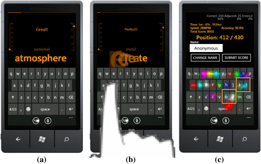
Fig. 1. Screenshots of Text Text Revolution: (a) Sample text users are instructed to type; (b) Letters exploding when users touch an expected or adjacent key; (c) End screen highlighting areas for improvement.
