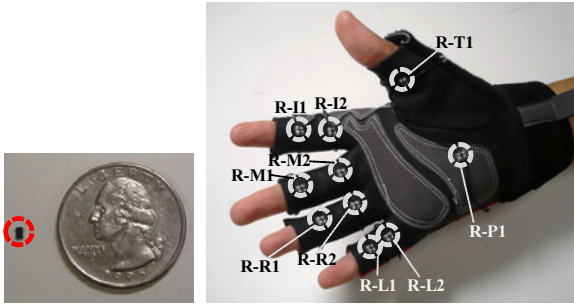
Fig. 2. A magnetic sensor shown next to a quarter dollar coin (left) and our prototype sensor glove (right). We provided each sensor on the glove with an identifier. The identifier is labeled with an initial letter indicating the left or right hand, an initial letter showing its position, and a serial number. For example, the identifier of the first sensor attached to the little finger of the right hand is R-L1.
