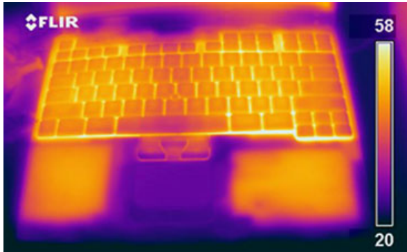
Fig. 2. Infrared image of a notebook computer with plastic surface when the underside heaters are activated. Temperature scale is in degrees Celsius.
