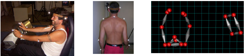
Fig. 10. Marker position (lateral view, back view) and 3D reconstruction (top view during driving)
