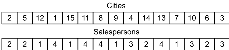
Fig. 5 Example of two chromosome representation for a 15 city mTSP with four salesperson [9].
