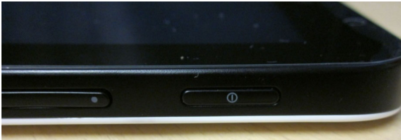
Fig. 2. Samsung Galaxy Tab Side View Showing Power Button Location and Label
