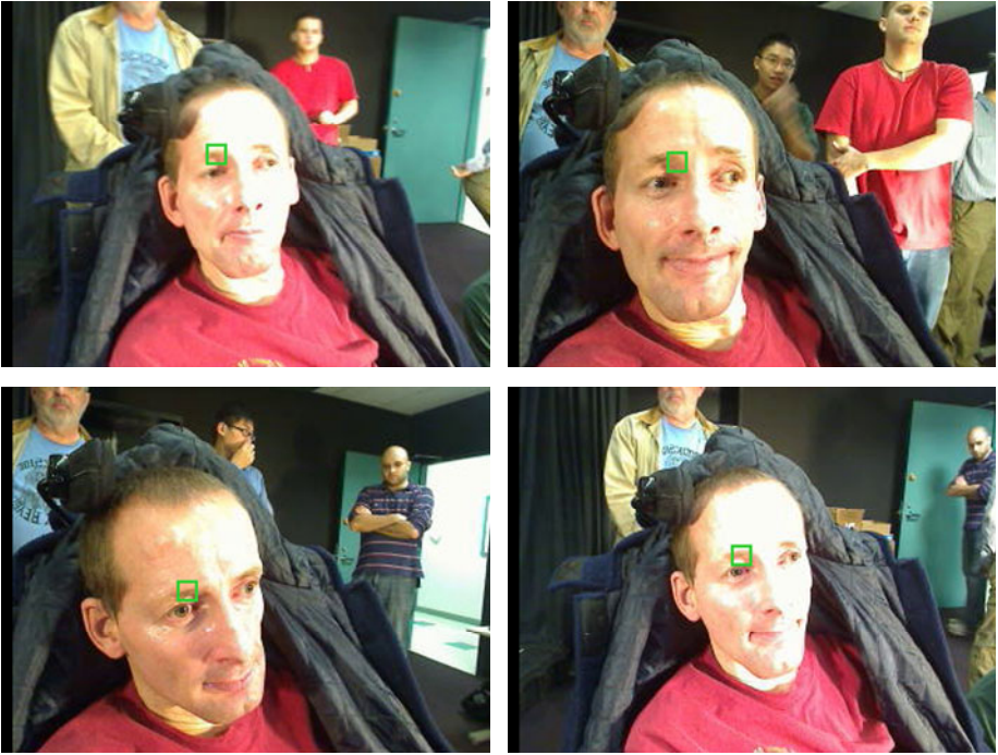
Fig. 3. Images of user interacting with system. The user can control the position of the mouse pointer with head motion. The green square indicates the tracked region, whose center is converted to a mouse pointer position on the screen.
