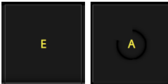
Fig. 3. (a) The border for “E” is highlighted showing the eye-over effect, and (b) the circle shows the selection in progress (See text for details.)
