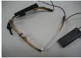
Fig. 4. Constantly wearable small see-through type HMD
