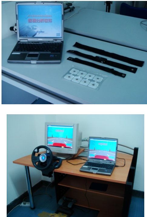
Fig. 1. The KF2 dynamic multi-parametric physiological detector and driving simulator
