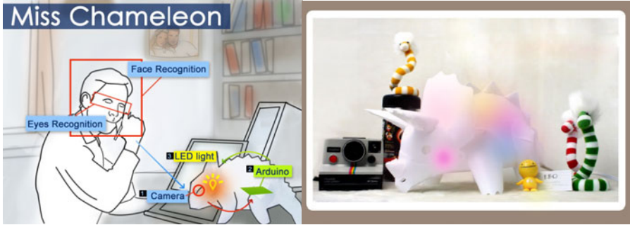
Fig. 2. Prototype I: Intelligent appliance with camera embedded inside (detect facial expression)
